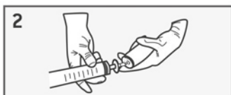
insert the syringe-filter assembly on the adapter mounted on the canister
