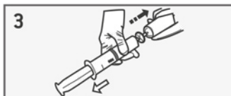
push the syringe against the canister to fill it with an adequate amount of gas
