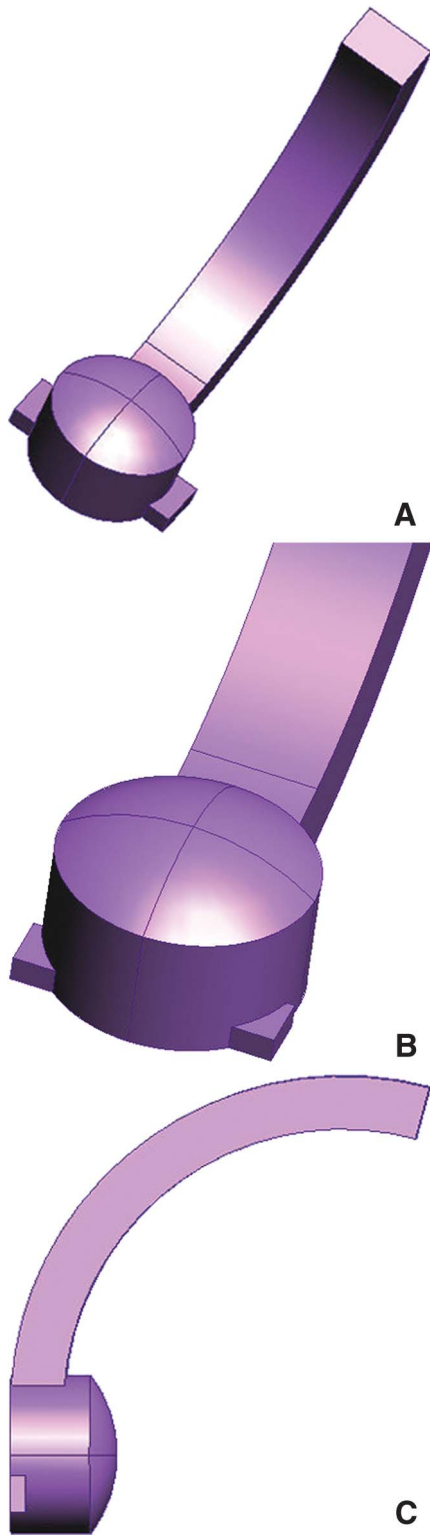
Fig. 1. The AMB with its radial “handle” element and a rounded “macular plate” (A). Note the two winglets at the margins of the terminal plate, designed for convenient suture placement (B) and the rounded preshaped curvature of the handle (C), intended to allow a more regular radial indentation over the desired meridian.
